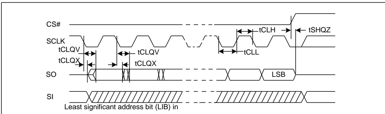
**Figure 80. Resume to Suspend Timing**
