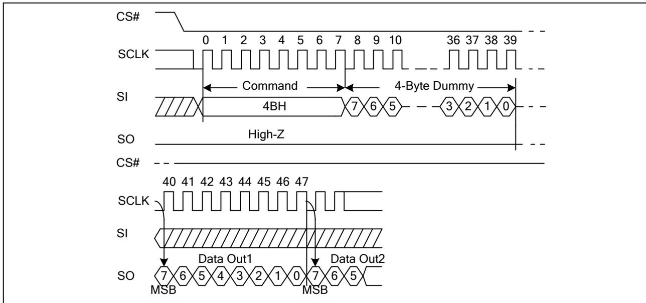
**Figure 55. Read Unique ID Sequence Diagram (ADS=1)**
